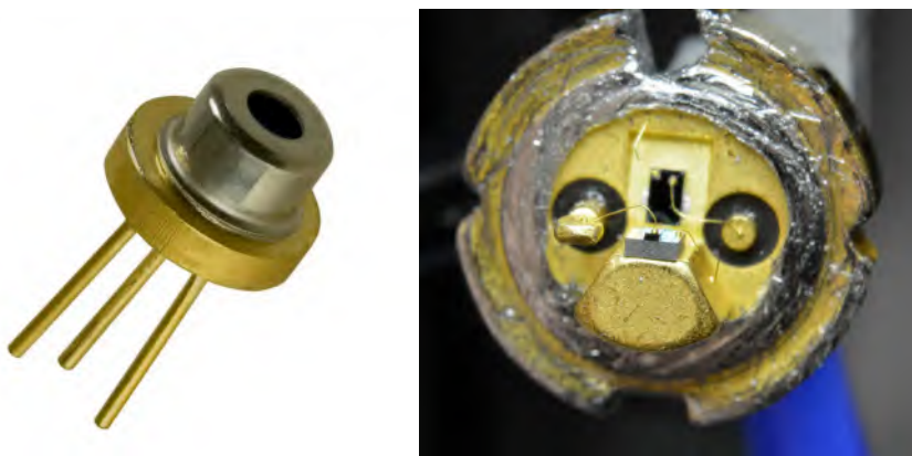
Figure 25: TO package laser with the cover cut away. Source: wikiwand.com
